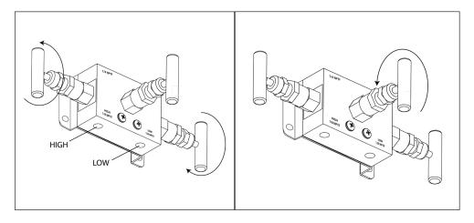
7 Open High and Low valves fully by rotating counter-clockwise
