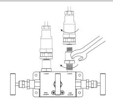
Detach the "Low" sensor from the cable (As shown in Step 3) Screw into the low port on the top of the manifold as marked. Re-attach cable.
