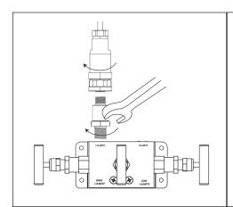
Screw sensor into the high port on the top of the manifold as marked. Re-attach cable.
