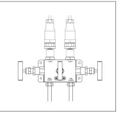
Attach High and Low pressure lines on the bottom of the manifold as marked.
