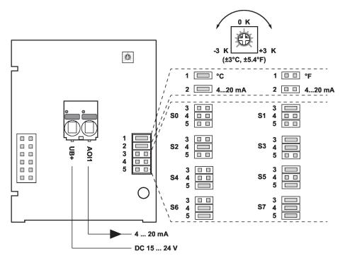
The following measuring ranges can be adjusted through the jumper settings:
