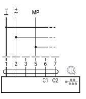
MP-Bus via 2-wire connection, local power supply
