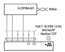
M-Bus with converter in parallel mode with BACnet/IP / Modbus TCP  $\,$
