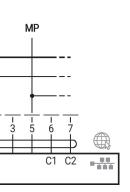
MP-Bus via 2-wire connection, local power supply
