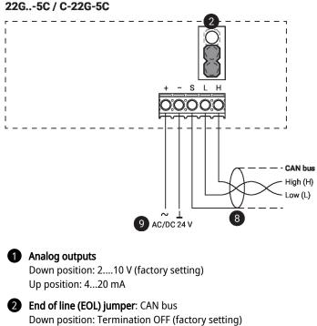
Up position: Termination ON (first and last unit only should have this jumper in the up position)
