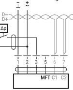
Switching contact requirements: The switching contact must be able to switch a current of 16 mA at 24 V accurately. Start point of the operating range must be parametrised on the MOD actuator as  $\geq 0.5$  V.
