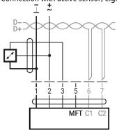
Possible input voltage range: 0...10 V Resolution 30 mV Connection with switching contact, e.g.  $\Delta p$  monitor
