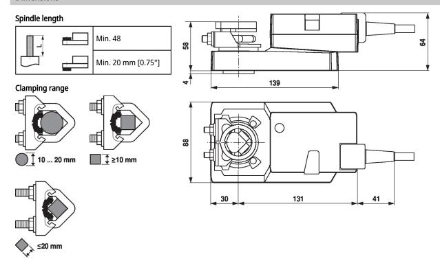
When using a round shaft made of CrNi (INOX): ø12...20 mm
