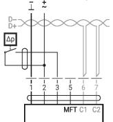
Switching contact requirements: The switching contact must be able to switch a current of 16 mA at 24 V accurately. Start point of the operating range must be parametrised on the MOD actuator as ≥0.5 V.
