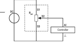
If the potentiometer is mainly operated in the same small angle range, we recommend wiring it as a voltage divider.
