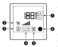
1 Temperature setpoint: Set the desired temperature
