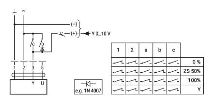
Override control with AC 24 V with rotary switch
