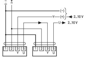
Control with 4...20 mA via external resistor
