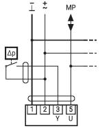
Max. 8 additional MP-Bus nodes • Switching current 16 mA @ 24 V
