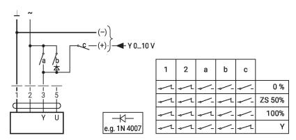
Control remotely 0...100% with positioner SG..
