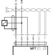
Possible input voltage range: 0...10 V Resolution 30 mV
