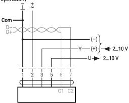
Connection with switching contact, e.g. Δp monitor
