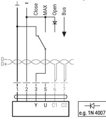
Modbus RTU / BACnet MS/TP with analogue setpoint (hybrid operation)
