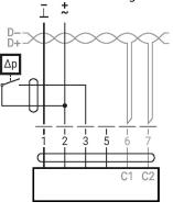
Switching contact requirements: The switching contact must be able to switch a current of 16 mA at 24 V accurately.
