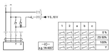
Control remotely 0...100% with positioner SG..
