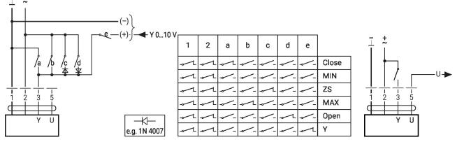
Override control and limiting with AC 24 V with rotary switch
