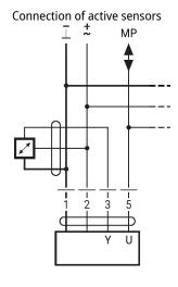
• Supply AC/DC 24 V • Output signal 0...10 V (max.
