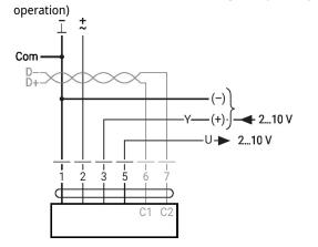
Modbus RTU / BACnet MS/TP with analogue setpoint (hybrid
