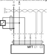
Possible input voltage range: 0...10 V Resolution 30 mV
