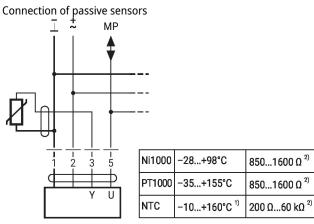
1) Depending on the type 2) Resolution 1 Ohm Compensation of the measured value is recommended
