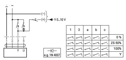
Control remotely 0...100% with positioner SG..
