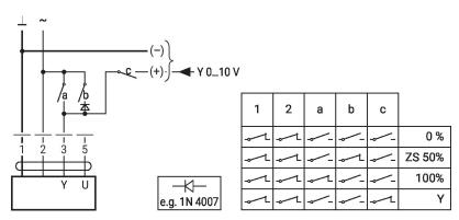
Control remotely 0...100% with positioner SG..
