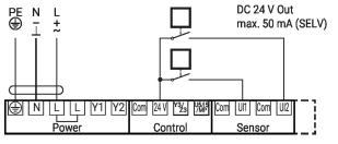
Connection of passive sensors (BACnet MS/TP / Modbus RTU / MP-Bus)
