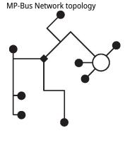
There are no restrictions for the network topology (star, ring, tree or mixed forms are permitted). Supply and communication in one and the same 3-wire cable • no shielding or twisting necessary • no terminating resistors required
