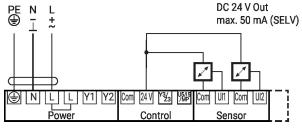
Switching contact connection (BACnet MS/TP / Modbus RTU / MP-Bus)
