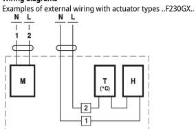
M = Actuator T [°C] = Thermostat H = Heating
