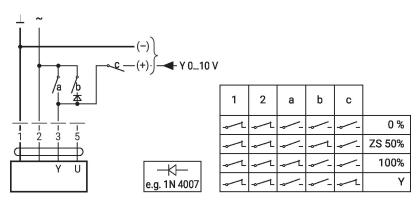
Control remotely 0...100% with positioner SG..
