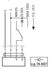
Control remotely 0...100% with positioner SG..
