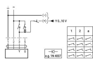
Override control with AC 24 V with rotary switch
