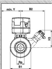
H1/X1: without spindle extension CQ L2: Maximum screwing depth.
