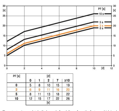
[d] = Power failure in days [s] = Pre-charging time in seconds PF[s] = Bridging time Calculation example: Given a power failure of 3 days and a bridging time (PF) set at 5 s, the actuator requires a pre-charging time of 14 s after the power has been reconnected (see graphic).
