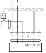
Switching contact requirements: The switching contact must be able to switch a current of 16 mA at 24 V accurately. Start point of the operating range must be parametrised on the MOD actuator as  $\geq 0.5$  V.
