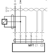
Possible input voltage range: 0...10 V Resolution 30 mV
