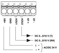
The following measuring ranges can be adjusted through the jumper settings:
