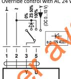
Control remotely 0...100% with positioner SG..
