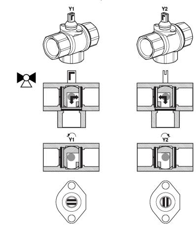
Flow setting At the actuator the end stop clip has to be removed in order to get the angle of rotation of 90°, which is needed for the change-over functionality.
