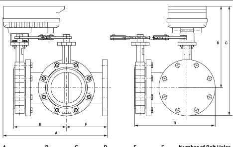
Valve with PR Actuator
