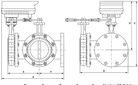
Valve with PR Actuator
