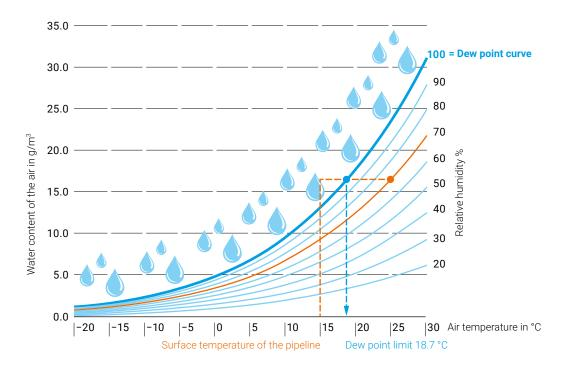
Condensation forms on cold surfaces when the dew point curve is exceeded. It is, therefore, necessary to insulate the pipeline to prevent condensation. See following comparison example.
