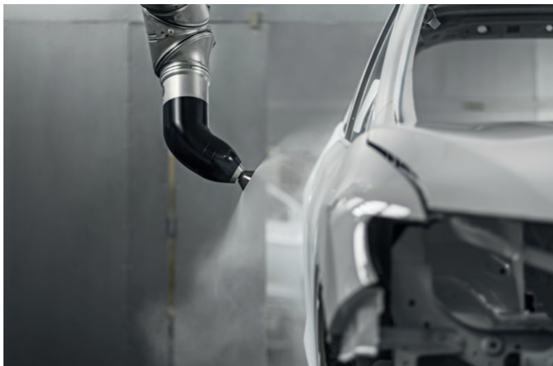
Automated painting process in the automotive industry
