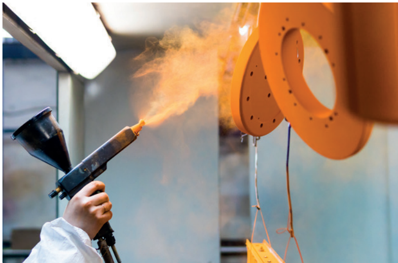
Powder coating process in paint shops
